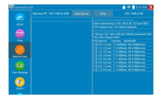
Or use tester as a Server, computer as test Client (select Client, input tester's IP address to test)
