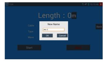
**Application:**TDR test is used for pulse reflection method, to transmit pulse signal for tested cable, when cable is open circuit or short-circuit, reflected pulse is generated, the tester receives and deals with the reflected wave, measurement results displayed on the screen. TDR can test cable open circuit and
