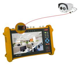
Note:1) If the IP camera requires PoE power, then connect the IP camera to the tester's LAN port. The tester will supply PoE Power for the IP camera. Click on the icon labeled POE to turn the PoE Power off or on.
