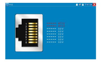
Connect a network cable from a PoE switch to the tester's PSE IN port. Connect an IP camera or other PoE using node to the tester's LAN port, the PoE voltage and the cable's pin connection status show on the screen.
