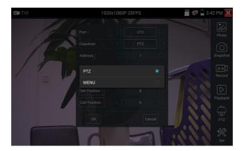
Input calling dome camera menu address code, after finishing the parameter settings, you can press the key (ENTER) or click the icon to call the dome camera menu.
