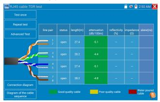
**Advanced Test:** test cable pair status, length, attenuation, reflectivity, impedance, skew and other parameters.
