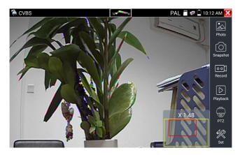
If not use touch screen to operate, press the key (TELE+) to zoom out, press the key (WIDE-) to zoom in, press upward and downward key to move the image.
