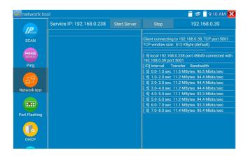
Network bandwidth testing can also be tested with a computer using compatible network bandwidth testing software. Install network bandwidth testing software on a computer, as a test Client or Server, to do the mutual testing with the tester. If use computer as the server, the computer IP address is :192.168.0.39
