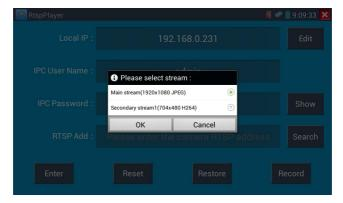
Note: In the event the Integrated Mount Tester does not auto detect the rtsp stream, refer to the specific camera manufacturer for the specific rtsp stream url. you may find this on line with a search of the camera model number and the word rtsp.
