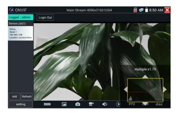
When the image is enlarged, if not operate on touch screen, it can operate by the keyboard ,press the key (TELE+) to zoon in , press the key (WIDE-) to zoom out ,press upward and downward key to move image.
