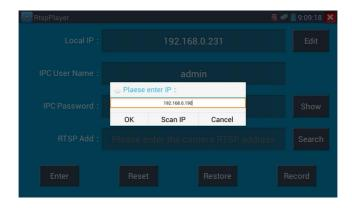
Local IP: This is the Integrated Mount Tester's IP address.
