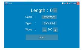
Built-in BNC cable, network cable, RVV control cable, Telephone line and TVVB cable etc can test, 11 groups user-defined cable can be set.
