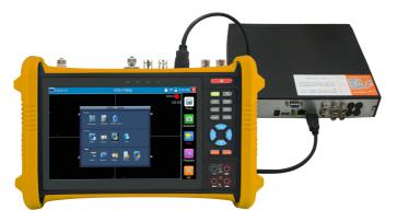
DVR or other device's HDMI in port connect to tester's HDMI in port, the meter will display input image.
