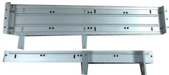
② Take off the bottom of the HDD bracket and CD-ROM bracket.
