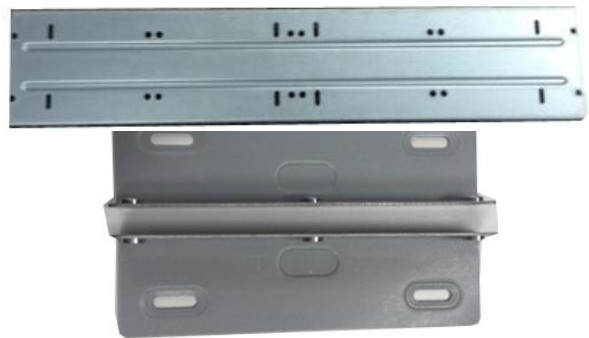
② Take off the bottom of the HDD bracket and CD-ROM bracket.
