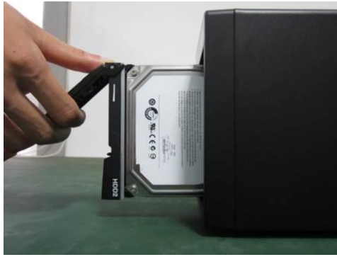
② Put the HDD to the HDD box at the front.
