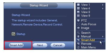
2. Click the Smart Add button. The NVR enables the DHCP function.
