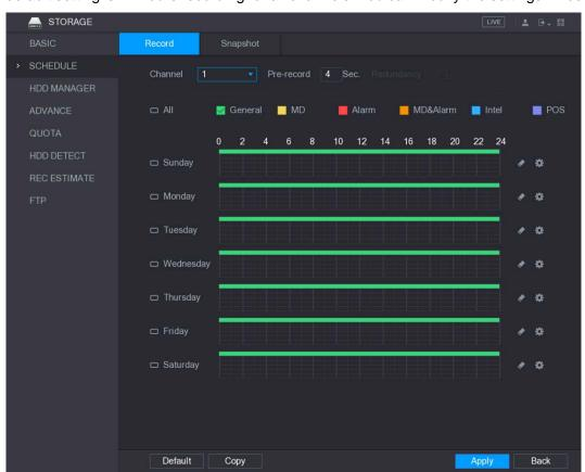
The default setting is 24 hours recording for all channels. You can modify the settings if needed.
