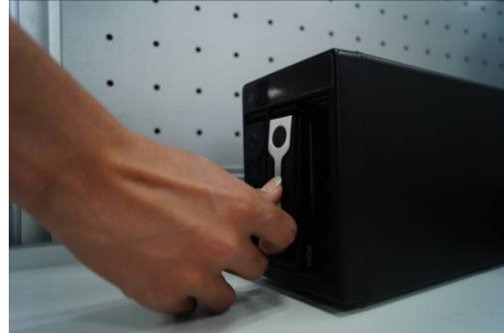
④ Put the knob back after you insert the HDD to the SATA board.
