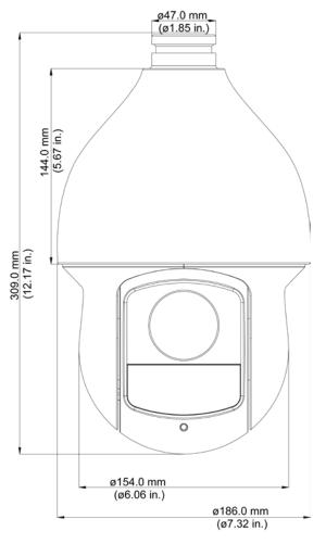
Figure 3-1: Dimensions for 59430IC
