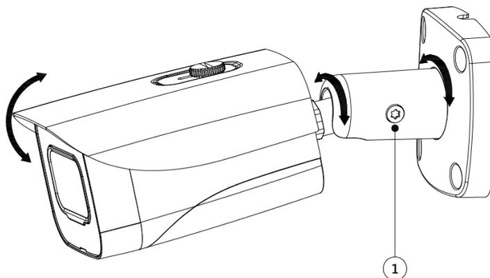
Figure 3-4 Lens adjustment (2)
