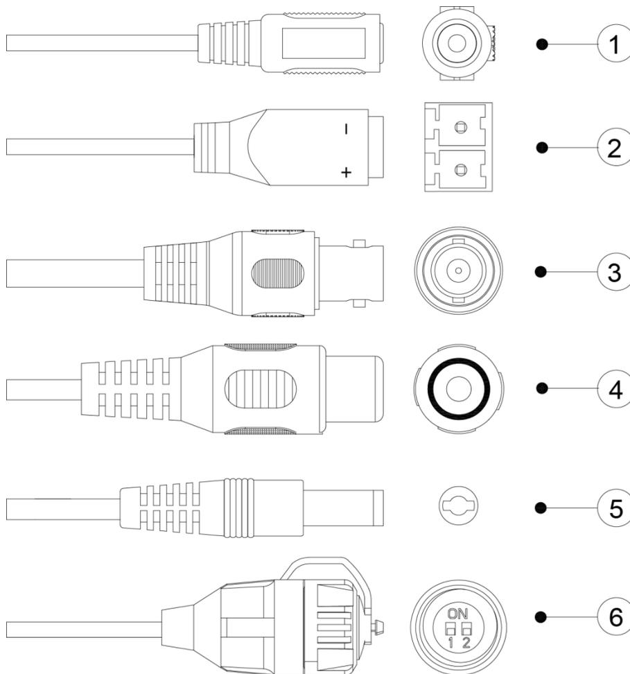
For more information about cable ports, see Table 2-1; for the operation method of ⑥ (DIP switch), see Table 2-2.
