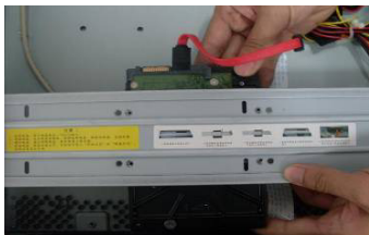
4. Line up the HDD to the four holes of the HDD bracket.
