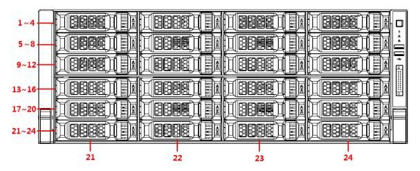
Figure 1- 4 Front Panel 4 (7024 with 24HDDs)
