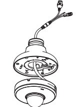
Figure 4-3 Pulling the speed dome cables
