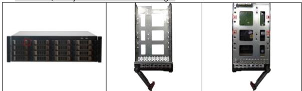
①Press the red button on the HDD box at the front panel, open the handle.
