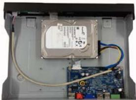
7. Align the upper housing with the clip and then place the cover back onto the NVR.
