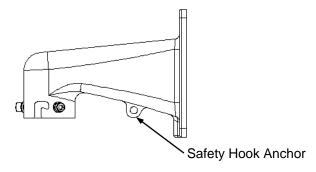
**Caution:** Make sure to attach the safety hook and ensure that it is securely fastened to the dome and to the wall mount to improve the safety and reliability of the installation.
