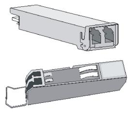
Figure 3-7 SFP module installation
