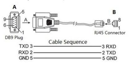
One end of RJ-45-DB9 cable is RJ-45 connector, which needs to be inserted into the console port of the device. And the other end is DB9 plug, which needs to be inserted into the computer controlling 9-pin serial port.
