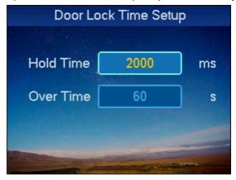
Step 2. Press (S) key to delete original data, input hold time and over time, press (OK) key.
