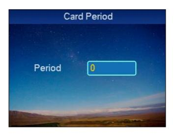
Step 4. Input time period, and press **[**OK]key. Input any number between 0~127. Screen displays period. See Figure 4-7.
