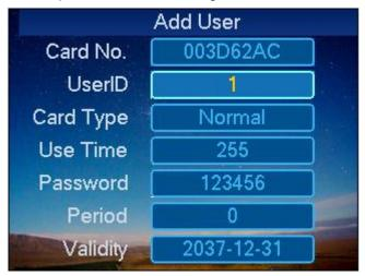
Step 3. Use key to input card no. or place card at swiping area to scan.
