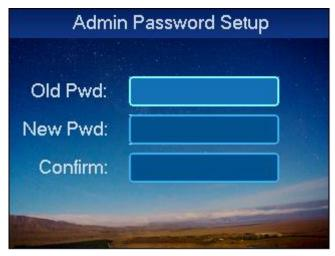
Step 2. Input old password, new password, confirm password, press 【OK】key.
