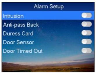
Step 2. Slect alarm to turn ON, and press 【OK】key as follows. Press 【OK】key again to close the alarm.
