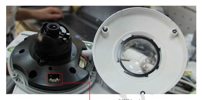
RS232 board connector port, Connect with RS232 board.
