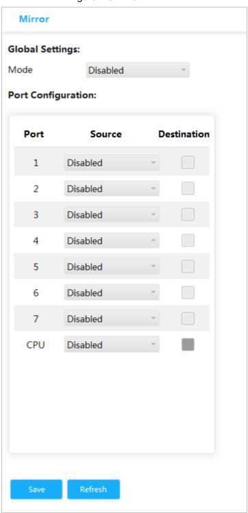
Step 2 In Global Settings, select Enabled in Mode to enable mirroring.
