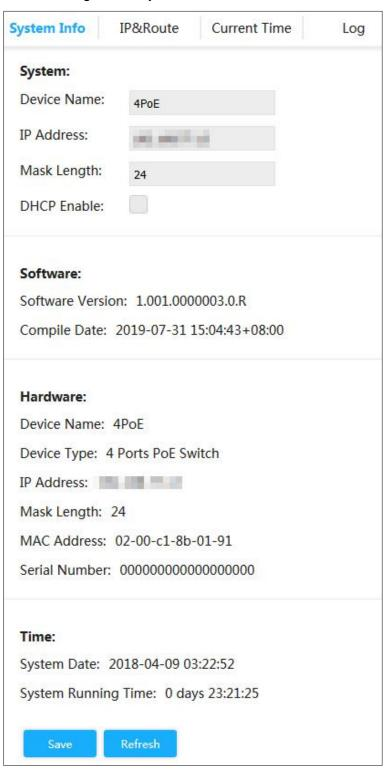
Step 2 Enter the device name, IP address and mask length and DHCP enable.
