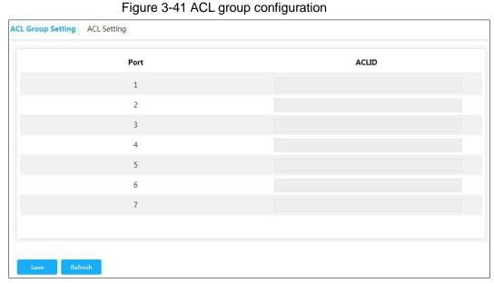
Step 2 Enter ACL ID. Ensure the ACL ID has been added during ACL configuration.
