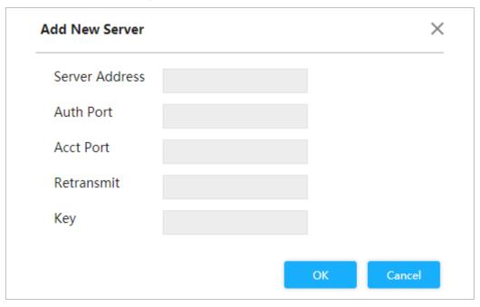
Step 3 Set the server address, auth port, acct port, restransmit and key.
