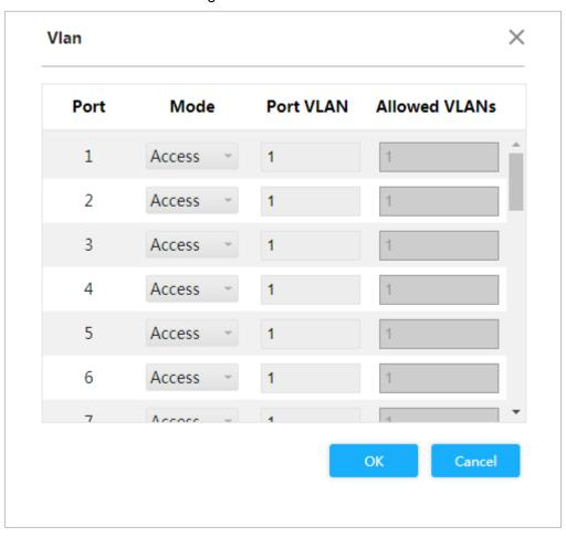
Step 2 Configure the port VLAN parameters. See Table 2-2.
