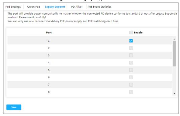
Step 2 Select the **Enable** box for the corresponding port.
