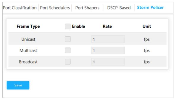
Step 2 The port can receive the rate up to 1024 fps. See Figure 3-62.
