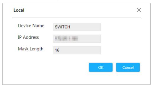
Step 2 Enter the system name, IP address, and mask length.
