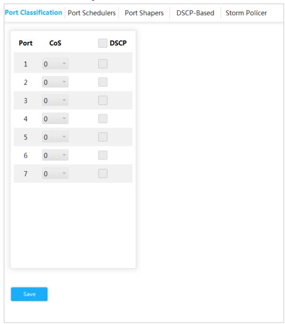
Step 2 Set CoS. For example: Set port 1 to be 1, and port 2 to be 2. See Figure 3-54. Port 1 and port 2 are ingress ports, and port 3 is egress port. The CoS value of port 2 is large than that of port 1, so the data of port 2 will pass port 3 first.
